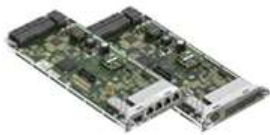
ETHERNET LIC WITH 1 COMBO AND 3 ELECTRICAL OR OPTICAL INTERFACES
